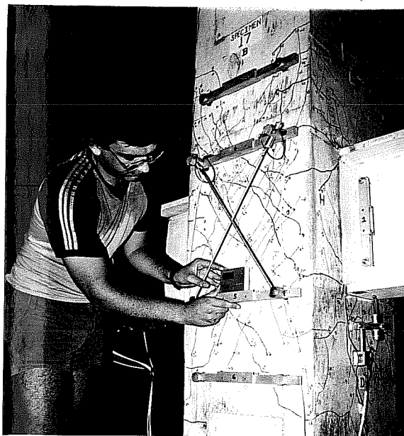
Fig. 2.11 Joint Deformation Instrumentation
